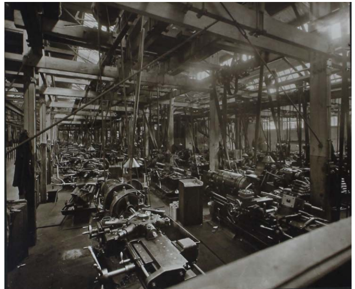
Revolver lathes at the Pelabon Munitions Works, East Twickenham, c.1915. © Guy Pelabon
